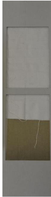
Figure 1: Photograph of the textile specimen mounted on the used specimen holders
